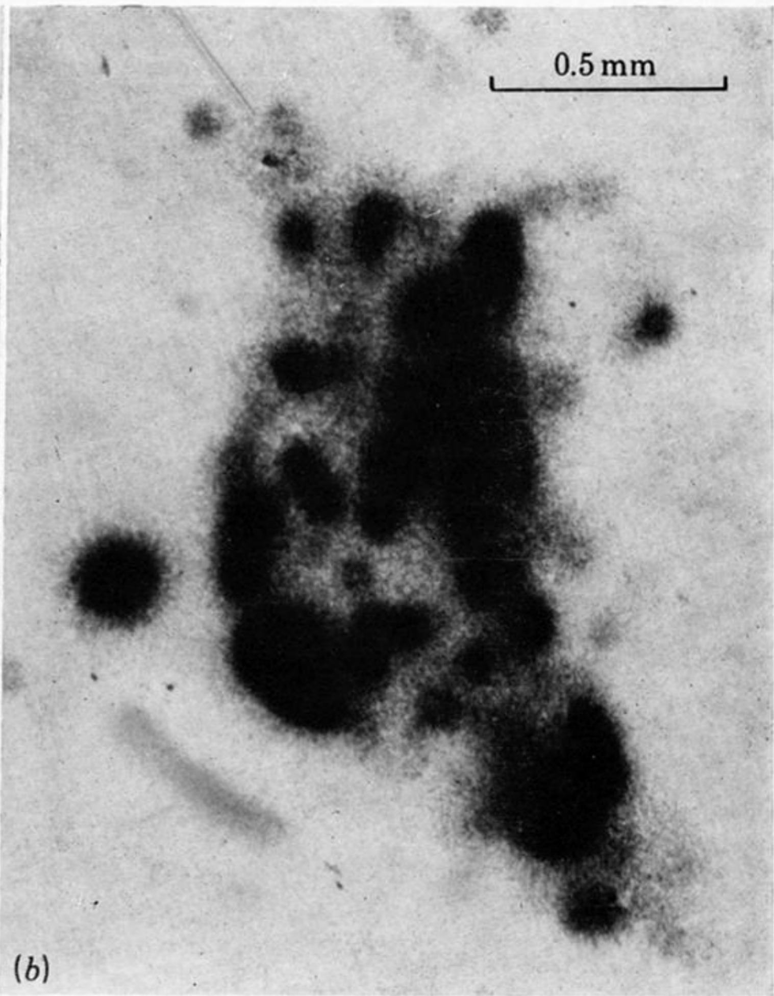
FIGURE 4. Uranium in zircon in primary biotite from Cairngorm. (a) Polished thin section; (b) lexan print showing fission track distribution.
